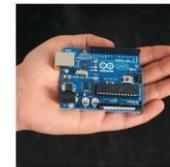
Arduino is an open-source electronics prototyping platform based on flexible, easy-to-use hardware and software, it's intended for artists, designers, hobbyists, and anyone interested in creating interactive objects or environments.
